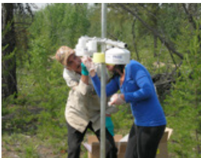
Figure 4: Fort McKay Elder Howard Lacorde assists WBEA technician Natalie Bonnell to change passive air filter
